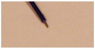
Now, "tin" (apply solder to) the end. The stranded copper will soak it up like a sponge. Be quick to avoid melting a bunch of the insulation.
