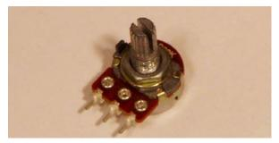
Now, tin the back of the pot in all three places (I've cut the pins off below):
