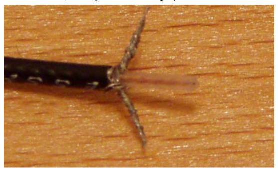
Cut the thicker group off. Strip enough of the *dielectric insulator* off to allow the *conductor* to fit through a hole on the PCB. Now, "tin" (apply solder to) the thinner group. "Tin" (apply solder to) the conductor:
