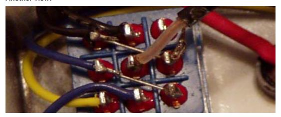
On the PCB side of the wire, cut back enough of the braid to prevent it from touching anything else on the PCB. Strip enough of the dielectric insulator off of the conductor to fit through the input hole. Solder. Done.
